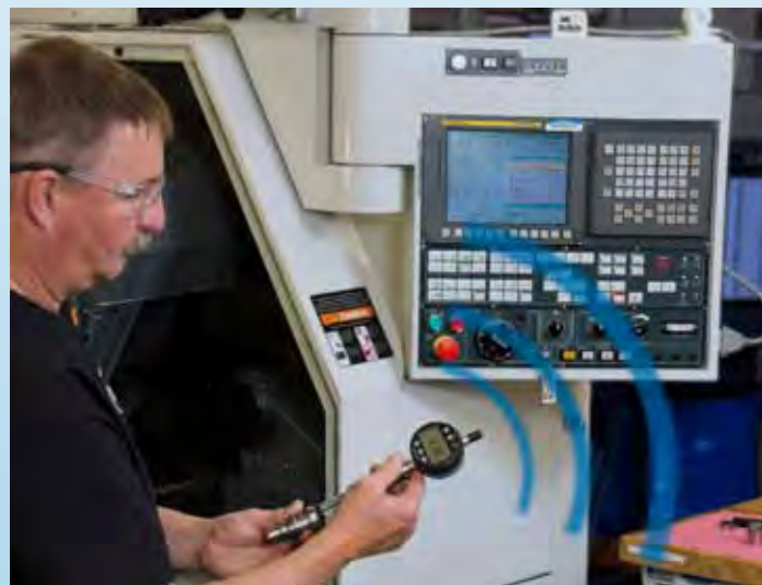
Wireless Bore Gaging on the Shop Floor
